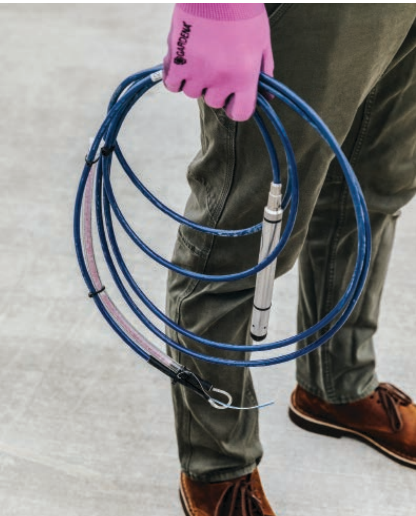
Kieran Fahey with a sensor used to measure water pressure and flow in South Bend's sewers.
